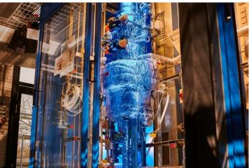
PU depolymerization and destillative purification of recycled PU inputs
