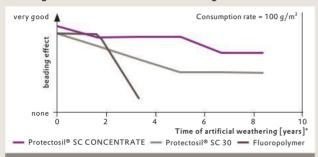
\*300 hrs. artificial weathering correspond to about one year outside weathering (conditions South-West Germany) This diagram shows the performance of various Protectosil® products.
