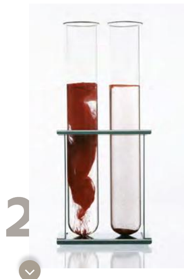
Self-dispersed red iron oxide treated with Dynasylan® 4148 (left) and untreated (right) after 20s in water
