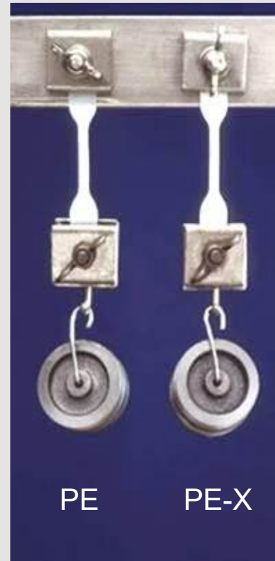
PE (non-crosslinked polyethylene) PE-Xb (silane crosslinked polyethylene)
