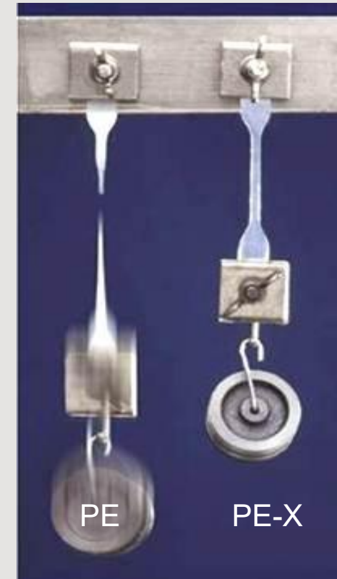
PE (non-crosslinked polyethylene) PE-Xb (silane crosslinked polyethylene)
