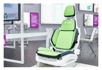
3D-printed prototype of a car seat: All components are made of the same class of plastics to facilitate mechanical recycling.
